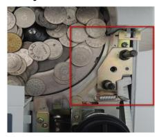
(4)After taking out the jammed coins, install back the thickness adjusting knob assembly part. There will be a sound of "ka" if the assembly part is installed to the right position.
