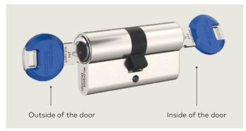
Key left in the lock? Not a problem! The double cylinder makes it possible to unlock the door from the opposite side with an authorised key when a key is inserted on one side and rotated in any direction. The inserted key turns with it. This function is guaranteed to work on both sides of the double cylinder.
