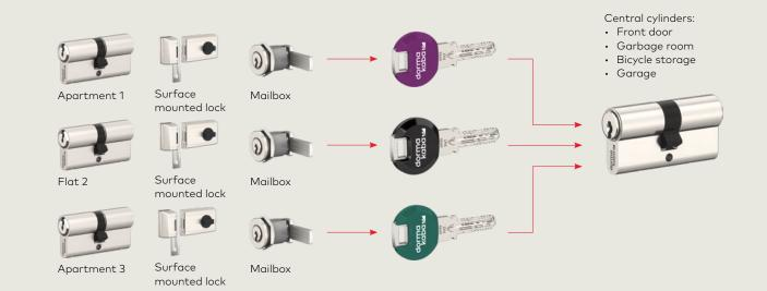
With the special **administrator master key system**, the main areas of several properties (i.e. several locking systems) in different locations can be closed with only one key (administrator key).
